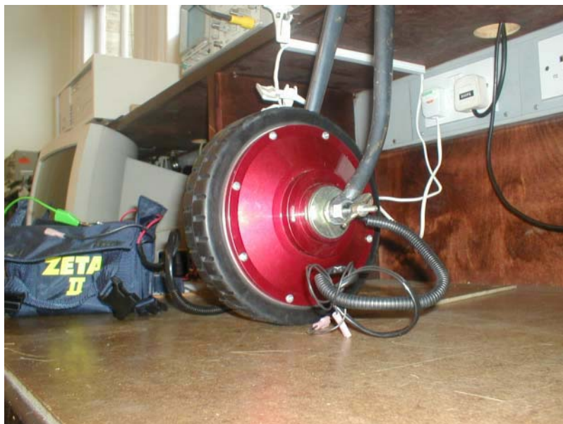
Fig 100 – Golden Island brushless hub motor fitted to chair (non-steering)
