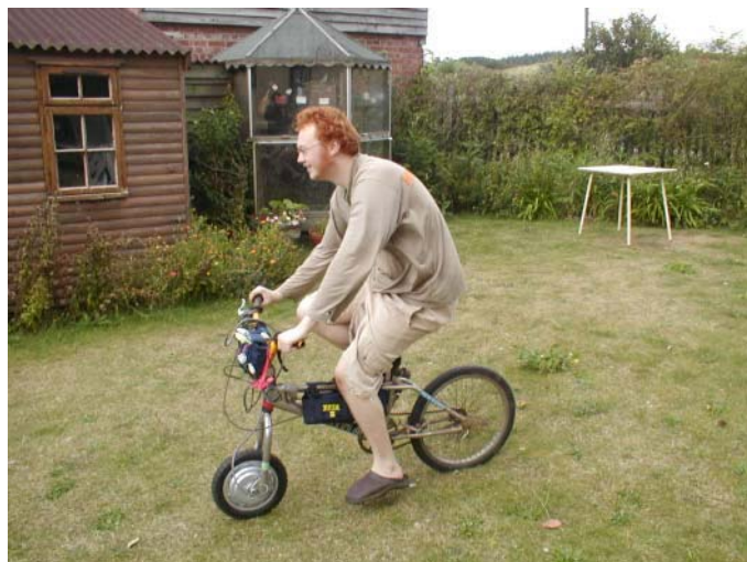
Fig 98 – Golden Island brushless hub motor fitted to bicycle
