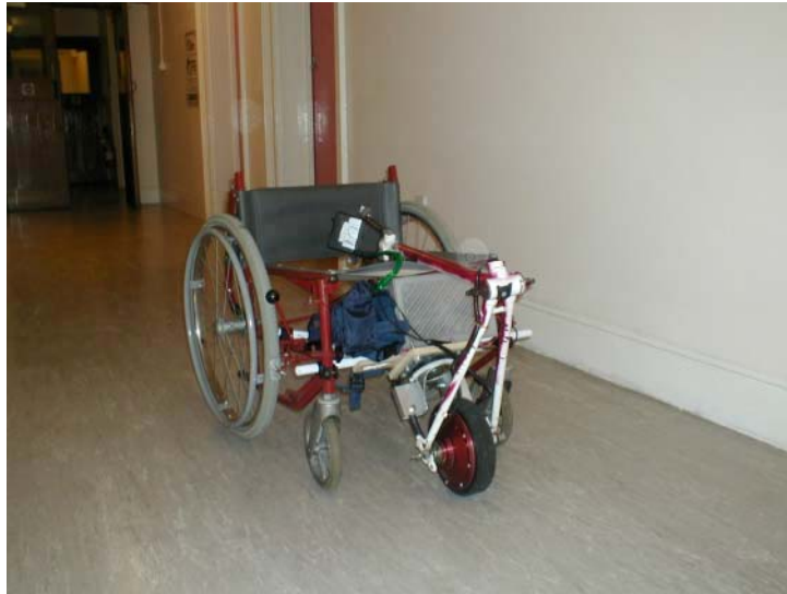
Fig 62 – Ultra-forward rake front wheel partial nutation steering prototype
