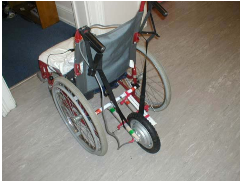
Fig 100 – Golden Island brushless hub motor fitted to chair (non-steering)
