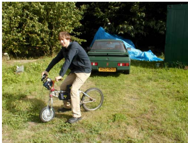
Fig 97 – Golden Island brushless hub motor fitted to bicycle
