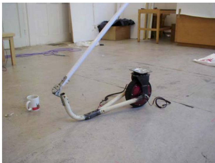
Fig 135 – Steering column with sprung hinge
