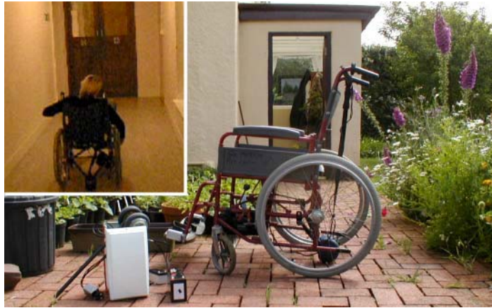
Fig 1 – A Sinclair drive unit fitted to the 8L chair to test whether hand braking of the pushrims was a feasible steering method
