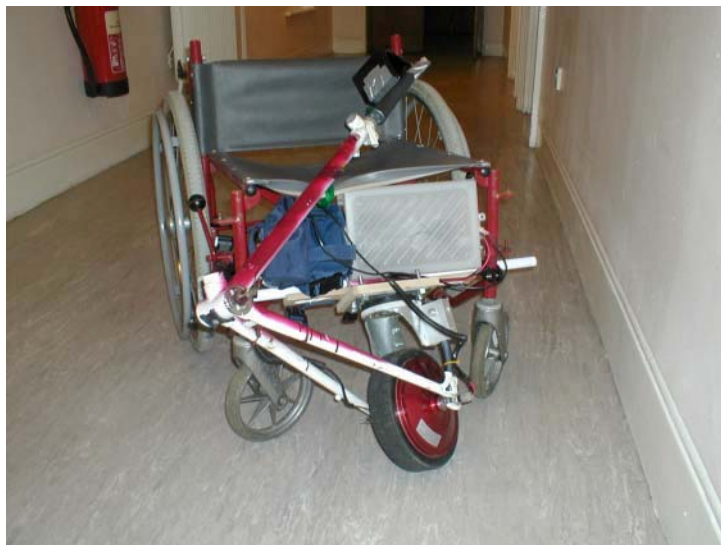
Fig 63 – Ultra-forward rake front wheel partial nutation steering prototype
