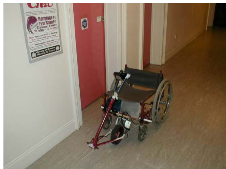
Fig 64 – Ultra-forward rake front wheel partial nutation steering prototype
