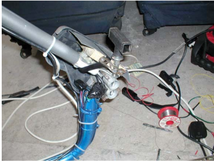
Fig 136 – Steering column with rolling hinge
