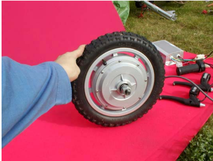
Fig 96 – Golden Island brushless hub motor
