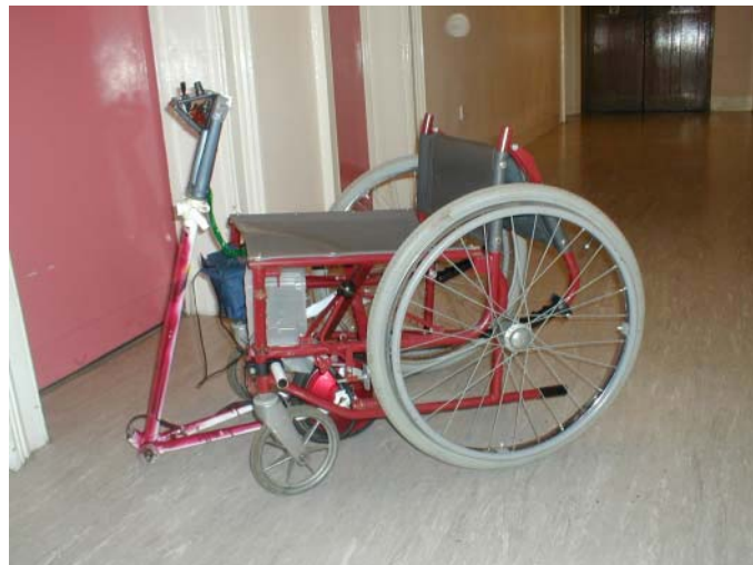
Fig 61 – Reverse-rake front wheel partial nutation steering prototype
